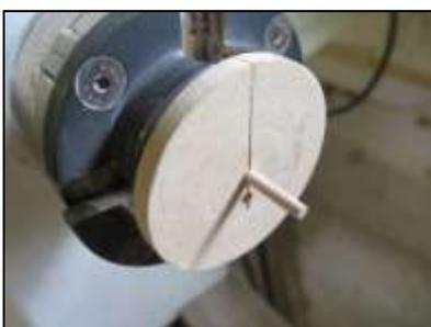
*I turn the beaks from a piece of 4mm beech dowel held in a pre-drilled disc as shown. The extra hole and length of band saw cut are deliberate and enable an excellent grip. I have a number of these 'collet' chucks with varying size holes for quickly gripping small items. The beaks are then cut to length and dyed yellow.*
