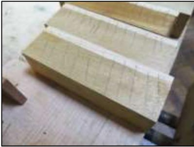
*When dry, the blank(s) are marked up to show where the surface needs sanding to achieve a flat surface.*
