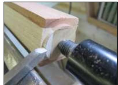
*I use a ring centre for preference, as I find that a lot less pressure is exerted on the blank for a positive location.*
