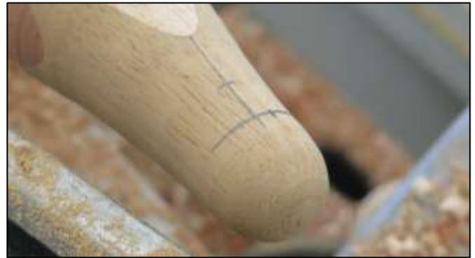
4 The position for the beak and eyes is carefully measured and marked out.
