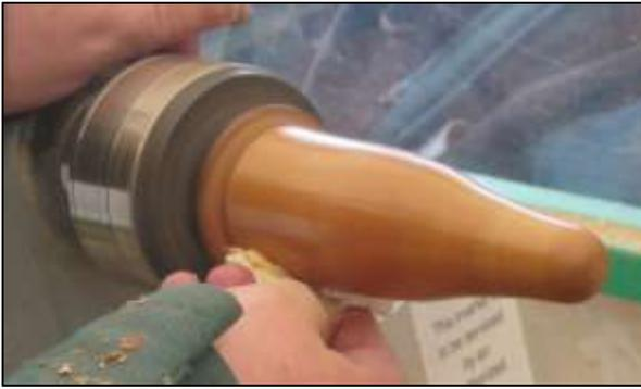
7 After sanding to 600 grit the penguin is finished with Friction Polish, and a coat of Carnuba wax.
