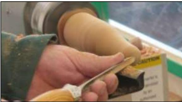
3 Most of the shaping is achieved with the spindle roughing gouge, but the spindle gouge is used to finish off the head.
