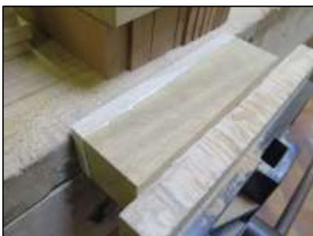
**PVA is nominally dry in 2 hrs, but takes 24 hours to fully cure. Given that the blank is going to be submitted to some fairly large shear forces on the lathe, please allow the full cure time between processes.**
