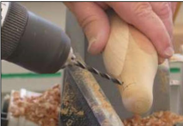
5 A spur point drill (4mm) is used for the beak, while a 3mm drill is used for the eyes. (if you use a 4mm for the eyes, they fall in!) Great care and accuracy needs to be achieved at this point, or the penguin will acquire the unfortunate name of Isiah.
